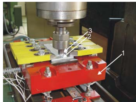
Figure 5. Research site: 1 - auxiliary equipment, 2 - work pieces of aluminum alloy 6082-T6, 3 - tool for FSW
