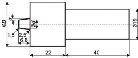
Figure 3. Tool with accepted dimensions and parameters D , d and \alpha
