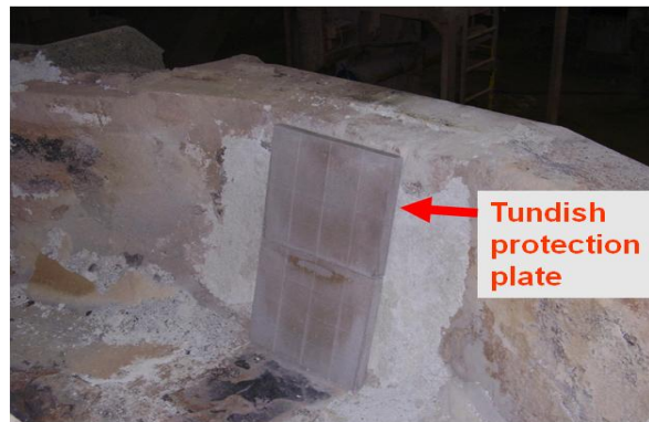
Figure 6. Protection of tundish front side, area of tundish working impact zone with installing of Ankoform protection plate. [5]
