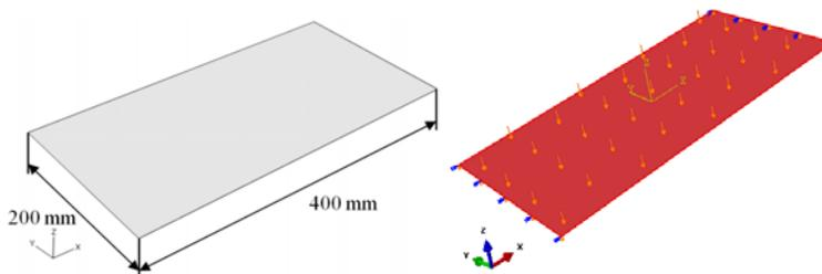
Figure 1. Plate geometry, loads and boundary conditions
