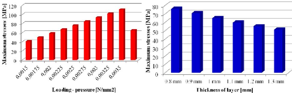
Figure 5. Variation of normal stresses with loading (a) and thickness (b)
