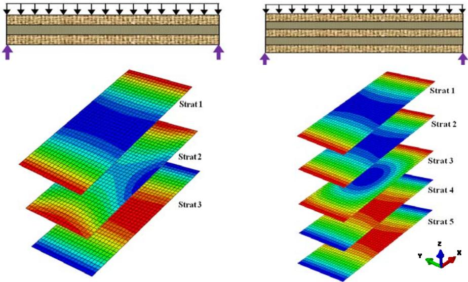
Figure 3. Distribution of normal stress on medium surface of each layer
