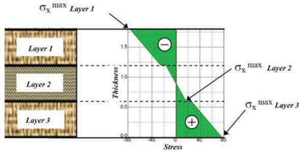
Figure 4. Distribution of normal stress  $\sigma_x$  related to composite thickness
