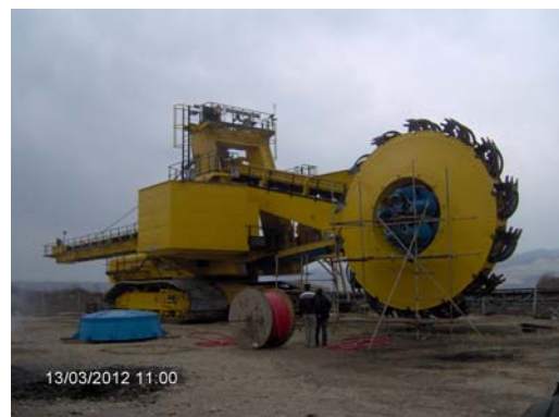
Figure 2. Excavator SH 630 after overhaul
