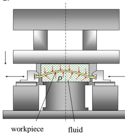
Figure 2. Sheet metal stretching by hydroforming
