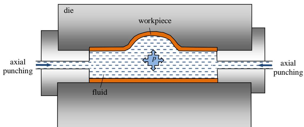
Figure 5. Hydroforming of tube
