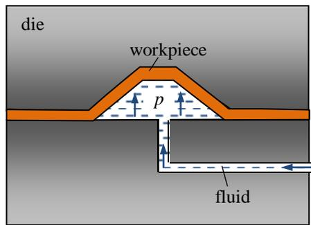
Figure 1. Sheet metal deep drawing by hydroforming
