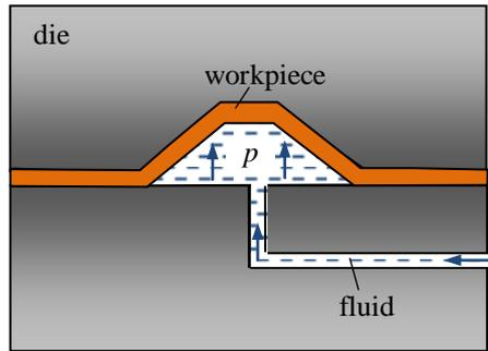
Figure 1. Sheet metal deep drawing by hydroforming
