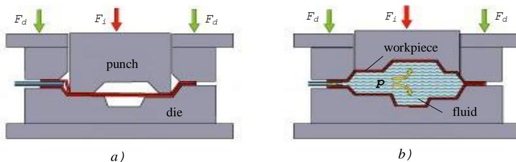
Figure 3. Hydroforming of welded sheet metal
