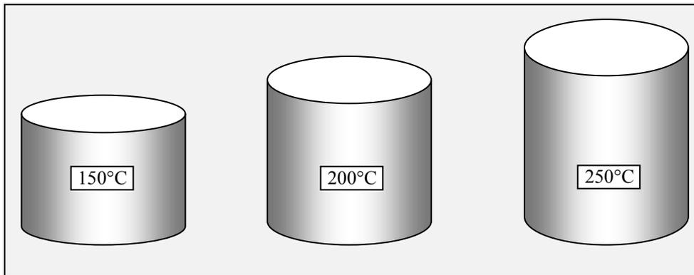
Figure 6. Parts formed by heated Hydroforming
