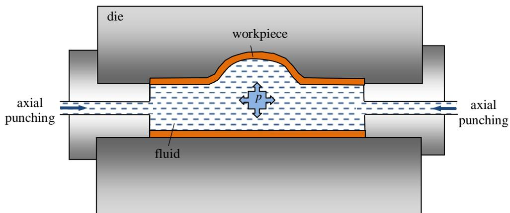
Figure 5. Hydroforming of tube
