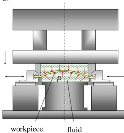
Figure 2. Sheet metal stretching by hydroformig
