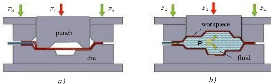
Figure 3. Hydroforming of welded sheet metal
