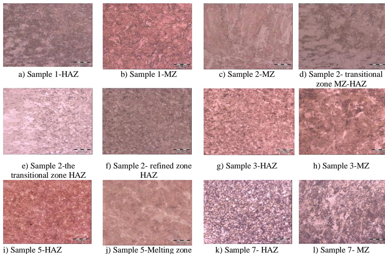
Figure 5. Microstructure of the weld nugget and heat affected zone[6] (Samples designated as in Figure 4)
