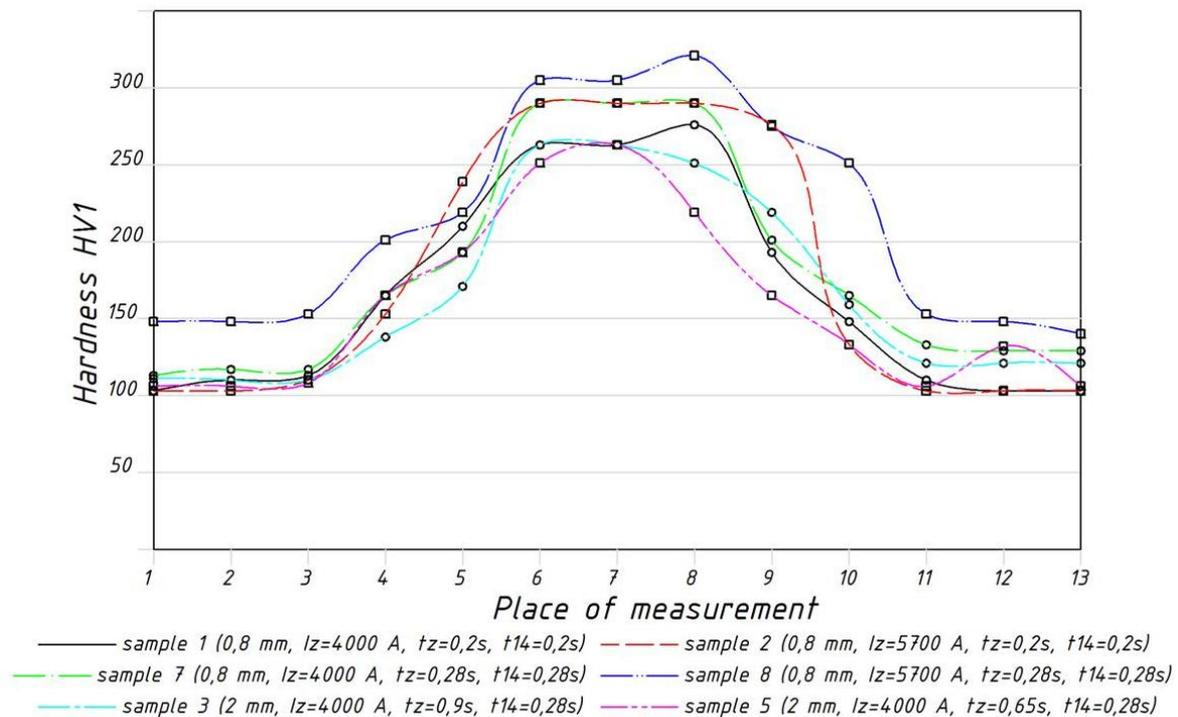
Figure 4. Hardness distribution in weld nugget and HAZ [6]
