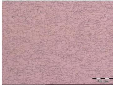
Figure 1. Microstructure of parent material
