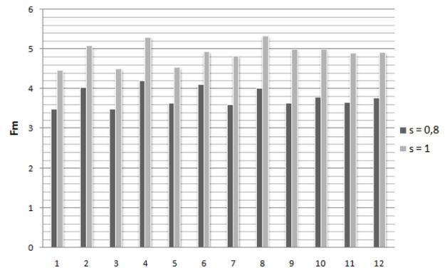
Figure 2. Weld strength for thicknesses 0,8mm and 1mm.
