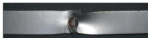
Figure 3. Failure of the weld
