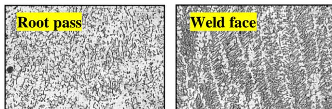
Figure 3. Microstructure of weld metal in ferritic - austenitic joint ( filler material Inox 29/9)
