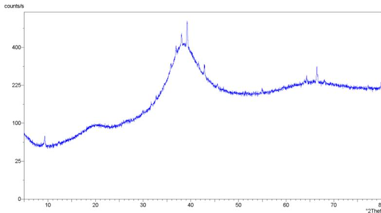
Figure 2. XRD intensity as a function of scattering angle for the partially crystalline  $Zr_{53}Cu_{40}Al_7$
