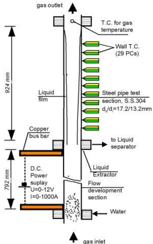
Figure 1. Experimental set-up for the heat and mass transfer studies into flue conduit
