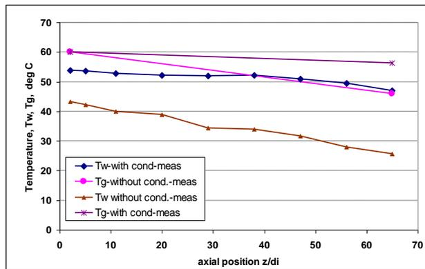
Figure 3 Comparison experimental wall and gas temperature for case II and case III
