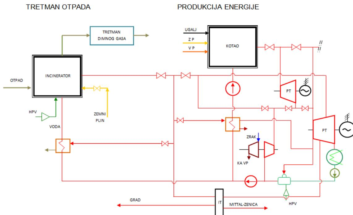
Figure 2: Proposed plant for thermal treatment of waste within the power station of the company by Arcelor Mittal - Zenica
