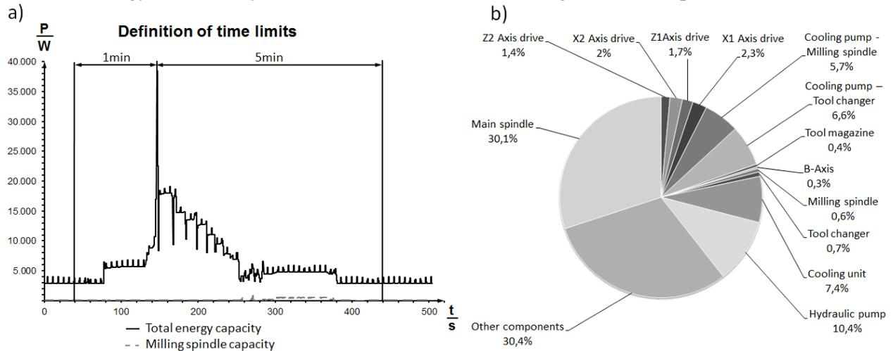
Figure 2: a) Total power consumption of the CNC lathe b) Energy distribution when manufacturing a test workpiece
