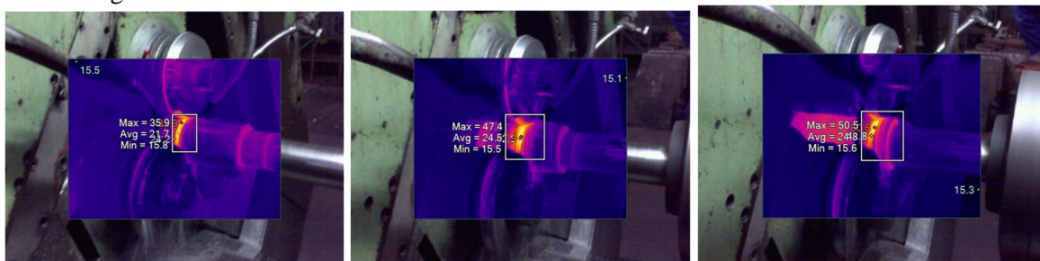
Slika 4. Characteristic positions (start, middle and end of the workpiece) for the determination of the temperature by processing of one sample from Al 99,5(Nr. 8) in the first processing stage [1]
