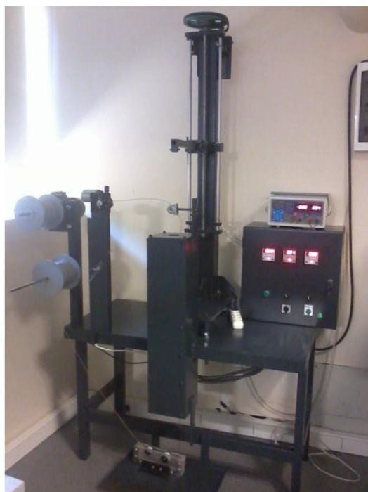
Fig. 1. The sol-gel coating system.
