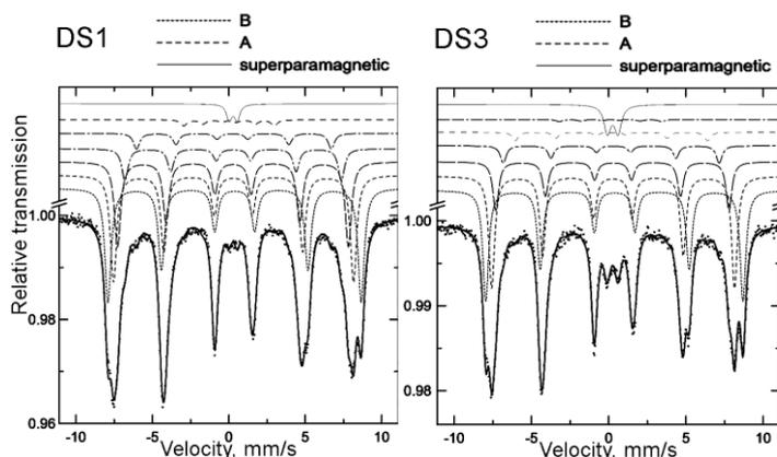
Figure 4. Mössbauer spectrums of the prepared Ni-ferrite powders
