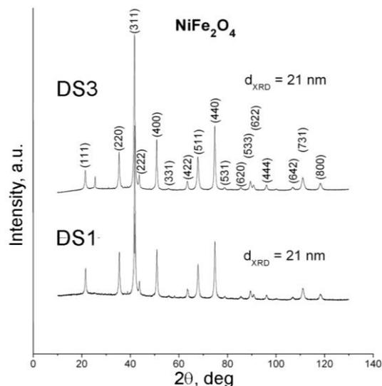
Figure 3. X-Ray diffractogram of the prepared Ni-ferrite powders
