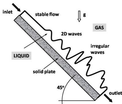
Figure 1. Liquid film flowing down an inclined solid plate.
