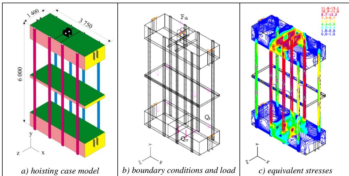
Figure 1. Hoisting cage model and structural analysis
