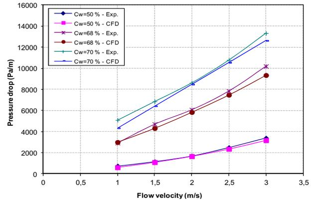
Figure 4. Comparison of numerical and experimental results of pressure drop in straight pipe of 42 mm diameter with flow velocity for mixture of fly ash and bottom ash
