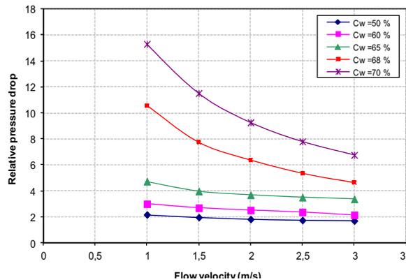
Figure 3. Variation of relative pressure drop in straight pipe of 42 mm diameter with flow velocity for mixture of fly ash and bottom ash (4:1) slurry
