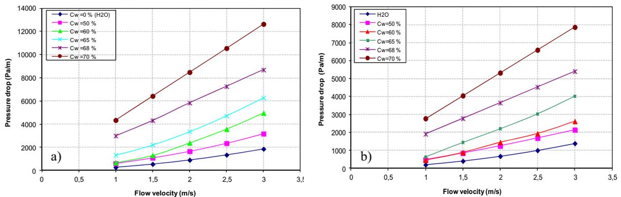
Figure 2. Pressure drop variation for mixture of fly ash and bottom ash (4:1) slurry with flow velocity at different concentrations (by weight) in: a) 42 mm and b) 53 mm, diameter pipeline
