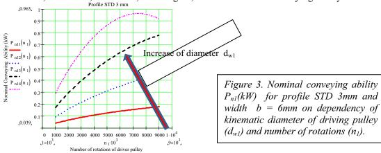
From the diagram shown in Fig. 3., can be seen that with increases in kinematic diameter of the driving pulley for the same number of rotations increases nominal conveying ability.
