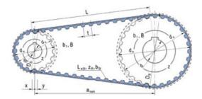
Figure 2. Transmitter with toothed belt.
