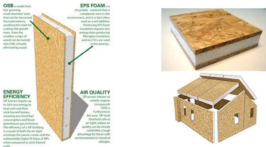
Figure 4. SIP paneli structural insulated panels
