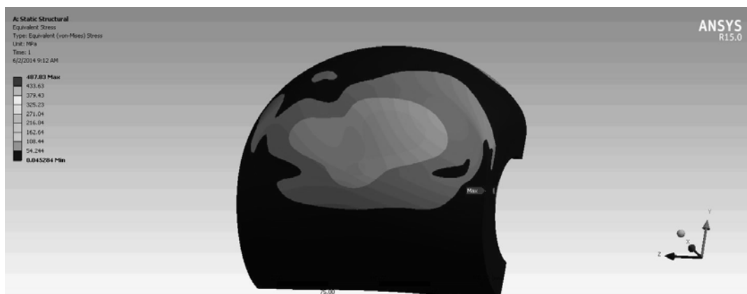
Figure 3. Equivalent stresses in the wall of the split sleeve – outer surface.
