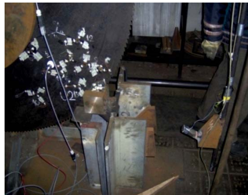
Figure 2. CSB with an impact pendulum, strain gauges and acceleration sensors
