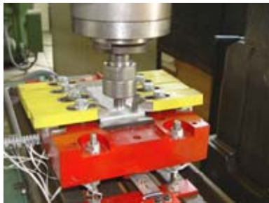
Figure 5. Machine performing FSW.
