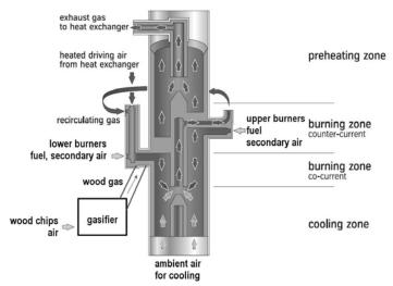
Figure 1. Annular shaft kiln for lime burning [4] with wood chips gasifier
