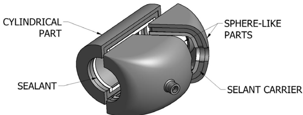
Figure 1. Split sleeve for branch connection repairs.
