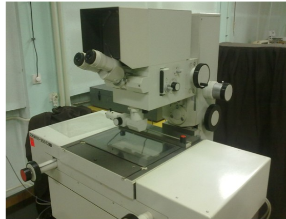
Figure 2. Measuring of top kerf width using a ZKM universal microscope
