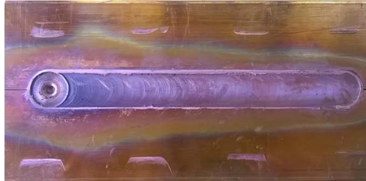
Figure 4. The appearance of the welded joint with the upper side of the welded workpieces
