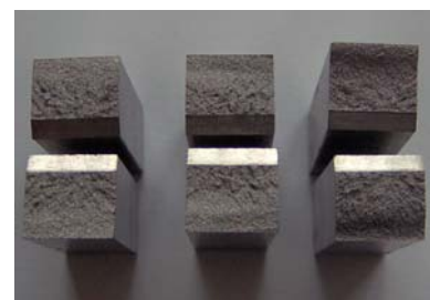
Figure 7. Reg. heat treated material 14MoV6-3 at 20 °C
