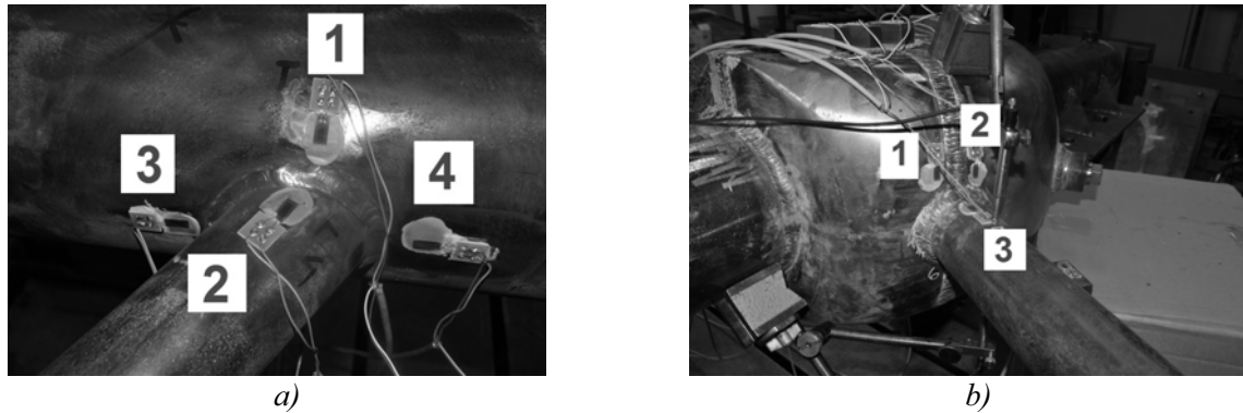
Figure 3. Position of strain gauges: a) strain gauges (SG) on the unreinforced branch connection (SG number 5 and 6 are on the bottom symmetrically with SG 1 and 2); b) strain gauges on the sample with split sleeve (SG 4 is placed symmetrically with SG 3)
