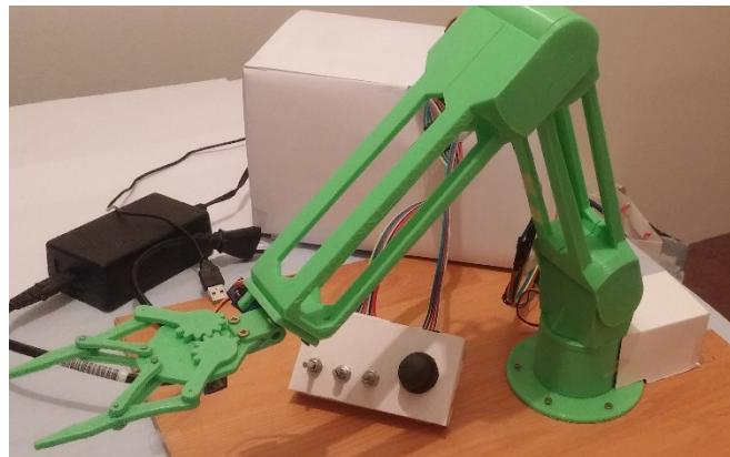
Figure 3. Actual system with local controls and power supply
