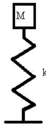
Figure 2. Oscillator, where M – plate mass; k – air stiffness.
