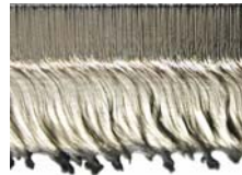
Figure 3b. Gas pressure too low
