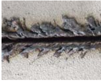
Figure 3a. Gas pressure too high, focus position too low
