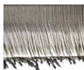
Figure 2a. Focus position too high
