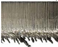
Figure 4a. Feed rate too low
