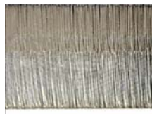
Figure 5. Optimal cut for steel AISI 314
